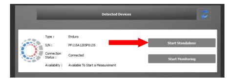
After that, the procedure described in the <u>start a measurement</u> chapter applies also to start a standalone measurement. After calibration results the software displays a success message confirming the switch of the Enduro device to the standalone acquisition
