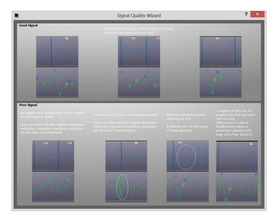
**Important:** The operator should check that heart cycles are detected (black lines slicing on a beat by beat basis the ECG waveform (red)). Similarly, please verify that fiducial points of the Z time
