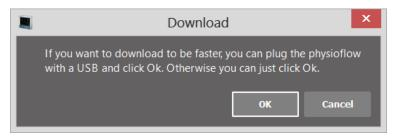
Bluetooth interface is selected by default to download the memory. To use USB interface, plug the USB cable before clicking the Ok button. Communication link selection is automatic and no configuration is required.
