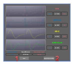
To compare time difference and value of two different points on the curve: click on any trend and maintain the click to set the first point and then move the cursor to the second targeted point. Release the button to obtain value of each point and the difference between the two. Time difference is common to all signals and is displayed on the bottom of the window. This procedure can be repeated as many times as necessary.
