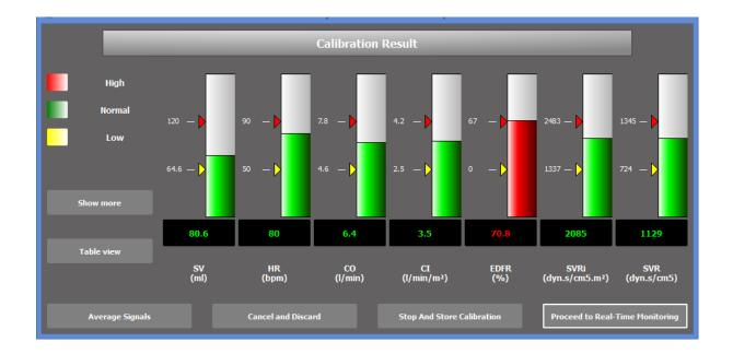
If the calibration results are satisfying click on the "Proceed to Real-Time monitoring" button to start acquisition. If no monitoring is necessary, but calibration must be saved for later review, click on "Stop and Store Calibration". If monitoring is not necessary, and the calibration results do not have to be saved, click on "Cancel and Discard.
