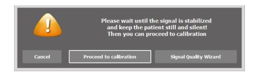
If users are not familiar with bioimpedance signal, the button "Signal Quality Wizard" provides help and illustrates the difference between good and bad signal:
